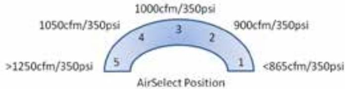
**QLX AirSelect is set at position 2 from the factory. DO NOT ATTEMPT TO ROTATE BELOW 1 OR ABOVE 5**
