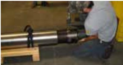
*Unscrewing the backhead. Use a lifting device or strap to support the backhead.*
