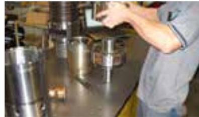
*Installing the valve cap.*
