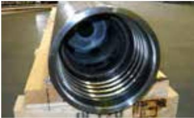
6. Pull the bit bearing from the hammer casing. Depending on the degree of rust or dryness in this area, a bearing puller may be needed for removal.
