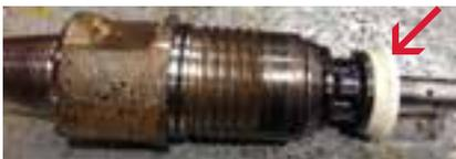
8. Inspect the bearing bore just above the internal flutes for wear using a telescopic bore gauge and micrometer. Replace the bearing if the net clearance between the bit and bearing is beyond the tabulated discard point. Replace the O-ring if it is worn or damaged.
