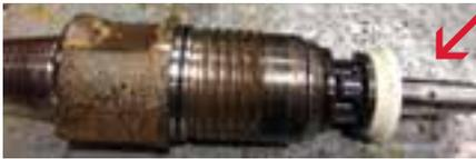
**Note for QLX 40:** If the valve assembly (item 7) is replaced with new O-rings, the valve should be installed in the closed position (valve seated against cylinder). This will insure that the hammer will start without incident. New O-rings may require a break-in period of 100 feet (30 meters).
