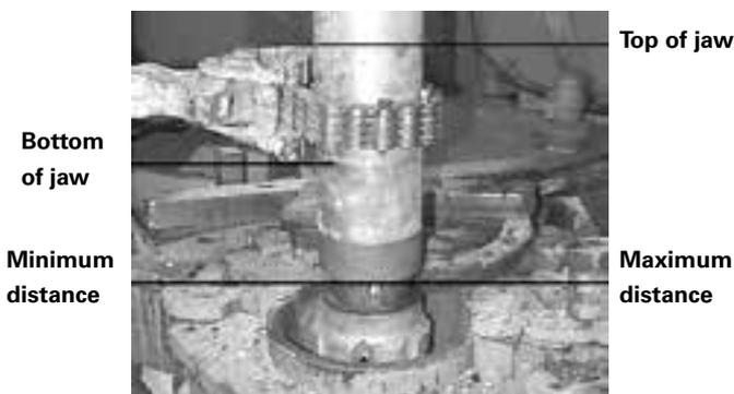
**QLX 35** minimum distance from bottom of chuck to bottom of jaw / 4.7 in. (119 mm). Maximum distance from bottom of chuck to top of jaw / 8,5 in. (216 mm)
