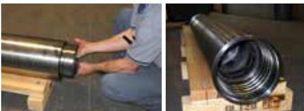
*Bit bearing installed.*
